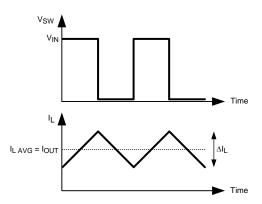
Figure 29. Switch and Inductor Current Waveforms
