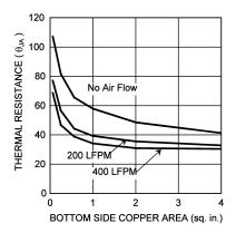
Figure 35. Thermal Resistance vs PCB Area
