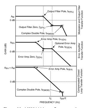
Figure 30. LM20144 Loop Compensation
